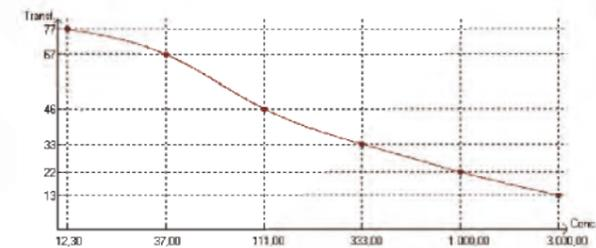
Standard curves can be stored and used for subsequent test runs as measured or adjusted by single or dual point calibration.
