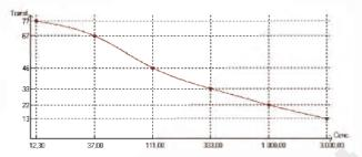
Standard curves can be stored and used for subsequent test runs as measured or adjusted by single or dual point calibration.
